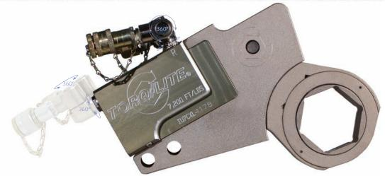
Inline ratcheting wrenches require minimum clearance while applying torque on the same plane as the nut, providing a marked improvement over square drive socket wrenches. Our patented design breakthrough reduced the overall dimensions of the inline ratcheting head allowing it to fit almost every application. Our IU-XL Series tool capacities range from 100 to 50,000 foot pounds of torque using a 10,000 p.s.i. hydraulic pump. "Extra light, dependable, and fits where others can not"
