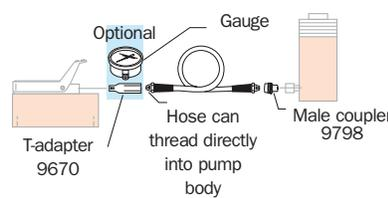
Air, Electric & Gas Pumps with valve system hook-up
